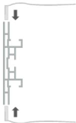
Place the textile print in the frame. Start with the corners and press the silicone strip in the channel.
