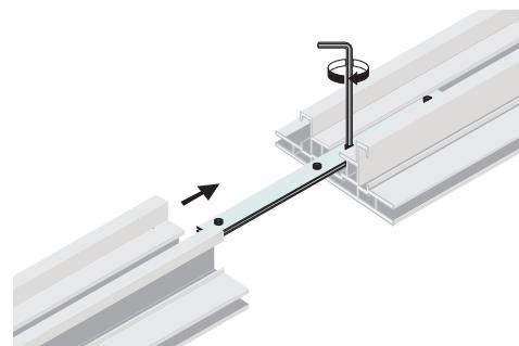
These extension sets can be placed in the channel where the frame is cut in half.
