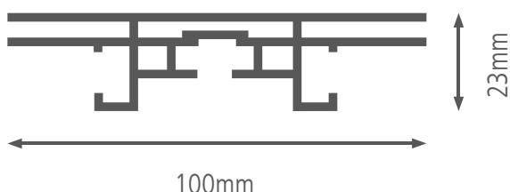
This aluminum profile is specifically designed for large format double-sided textile prints. With a smart design with multi-channel this profile is suitable for both standing and hanging.
