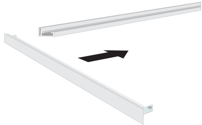
When connecting the frame, first place the lockset (FK-0210) without the punchholes, then the one with punchholes.
