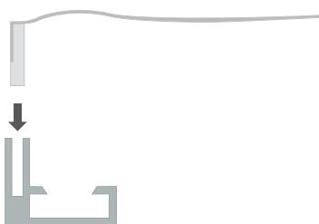
Place the textile print in the frame. Start with the corners and press the silicone strip in the channel.
