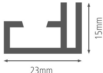
Single-sided aluminium textile frame, used for wall mounting. This is a very popular and widely applicable aluminum frame. This profile is usually mounted on the wall, in exhibition stands or interior integrated.
