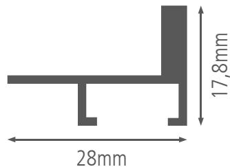
This aluminium profile is especially made for sheet materials. Simplicity and minimalism characterizes the L-shape 17,8.
