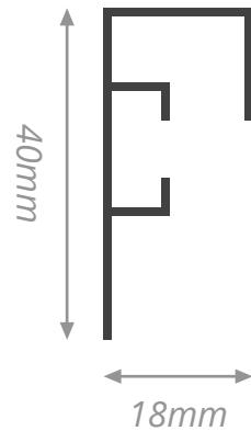
This aluminum profile is a frameless solution to let your print stand out. The profile is attached to the back of your sheet material, before mounting it to the wall. It lets the print float, which makes it perfect for a presentation of artwork in office, showroom or (art) galleries.
