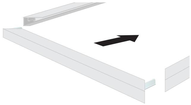
When connecting the frame, first place the lockset FK-0210 without the punchholes, then the one with punchholes.
