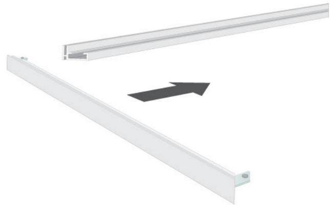
When connecting the frame, first place the lockset (FK-0210) without the punchholes, then the one with punchholes.
