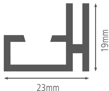
Single-sided aluminium textile frame, used for wall mounting. This is a very popular and widely applicable aluminum frame. This profile is usually mounted on the wall, in exhibition stands or interior integrated.
