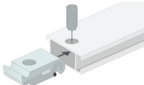
Then put the stabilizer (NF-04438) on the lockset, now tighten the screw with the delivered allen key.
