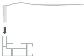
Place the textile print in the frame. Start with the corners and press the silicone strip in the channel.
