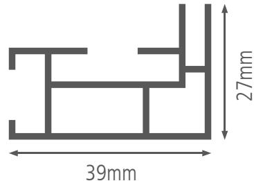
Single-sided aluminium textile frame, used for wall mounting. This is a very popular and widely applicable aluminum frame. With an extension set is any size possible. This profile is usually mounted on the wall, in exhibition stands or interior integrated.
