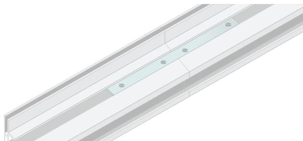
These extension sets can be placed in the channels where the frame is cut in half.
