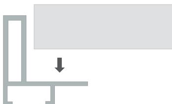
Place the print inside the frame. The montage is depending on the kind of material.
