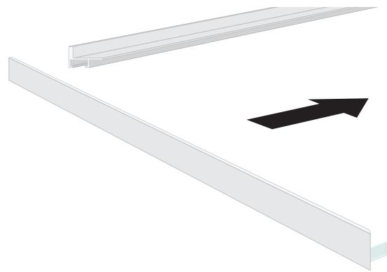
When connecting the frame, first place the lockset (FK-0210) without the punchholes, then the one with punchholes.
