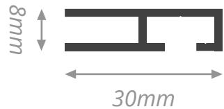
This single-sided textile frame is intended to be built into a niche, frame or cabinet to create custom made display solutions. This aluminium frame is used to finish off a niche, frame or cabinet. An ideal built-in solution.
