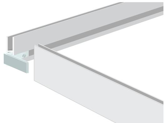
When connecting the frame, first place the lockset FK-0260 without the punchholes, then the one with punchholes.
