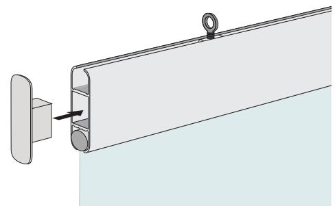
When the keder and ceiling mount are attached, place the endcap for the finishing touch.
