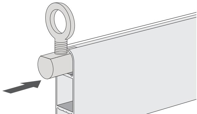
Apply the ceiling mount (FK-0609) into the groove of the frame.
