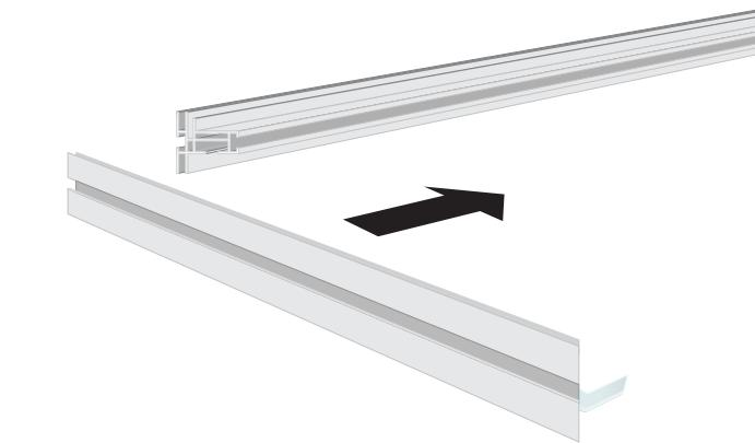
When connecting the frame, first place the lockset (FK-0200) without the punchholes, then the one with punchholes.
