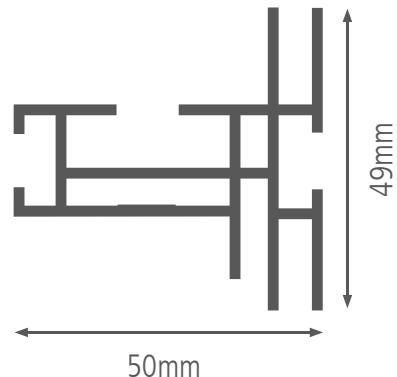
Double-sided textile frame, designed for freestanding and / or suspended use. This profile has a double channel, for placing two textile prints in the frame. Various accessories can be applied in a simple way. With the extension sets, every size is possible.
