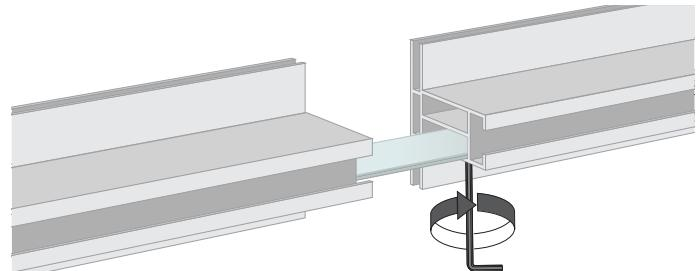
These extension sets can be placed in the channels where the frame is cut in half.
