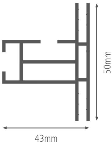
Double-sided textile frame, designed for freestanding and / or suspended use. This profile has a double channel, for placing two textile prints in the frame. Various accessories can be applied in a simple way. With the extension sets, every size is possible.
