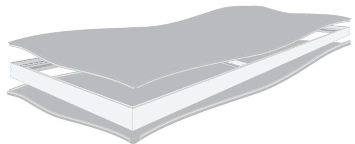
Place the textile print in the frame. Start with the corners and press the silicone strip in the channel.
