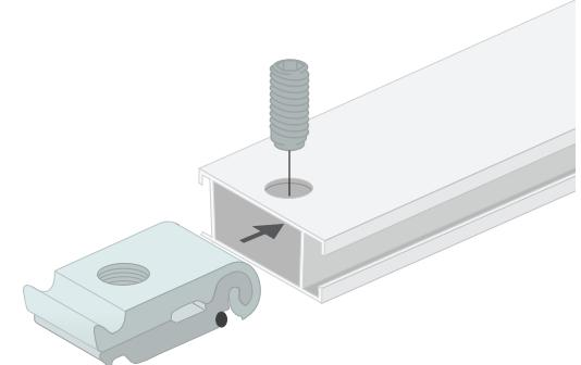
Then put the stabilizer (NF-04438) on the lockset, now tighten the screw with the delivered allen key.
