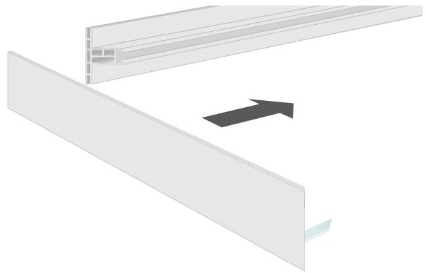
When connecting the frame, first place the lockset FK-0200 without the punchholes, then the one with punchholes.
