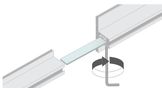
These extension sets can be placed in the channels where the frame is cut in half.
