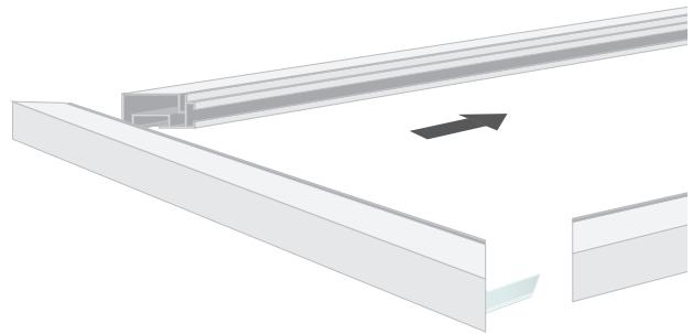
When connecting the frame, first place the lockset FK-0200 without the punchholes, then the one with punchholes.
