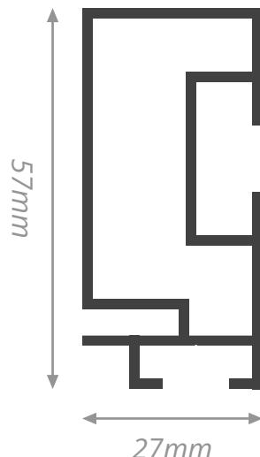
This single-sided and most strongest profile for the wall. Available in all colors. This aluminum frame is normally used in retail and office interiors or at public areas. The thick aluminum frame creates a modern eye-catcher.
