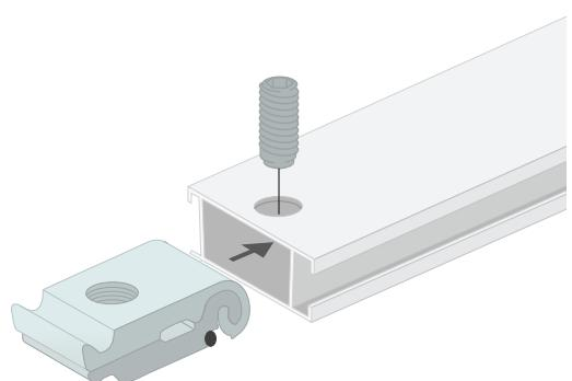
Then put the stabilizer (NF-04438) on the lockset, now tighten the screw with the delivered allen key.
